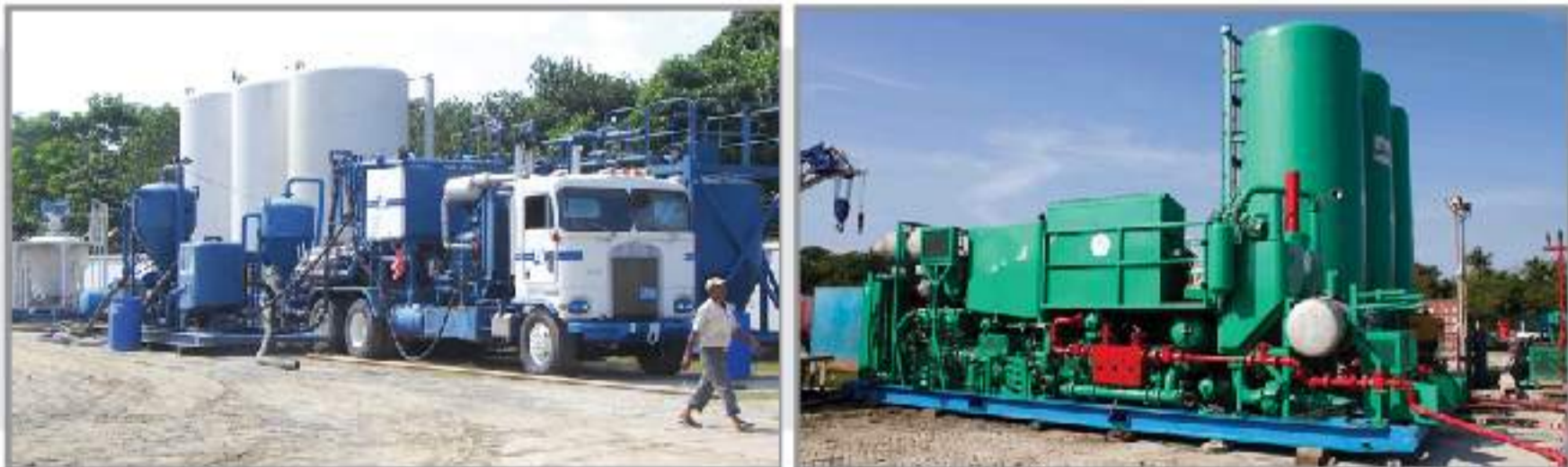
Cementing Units of BAPEX
