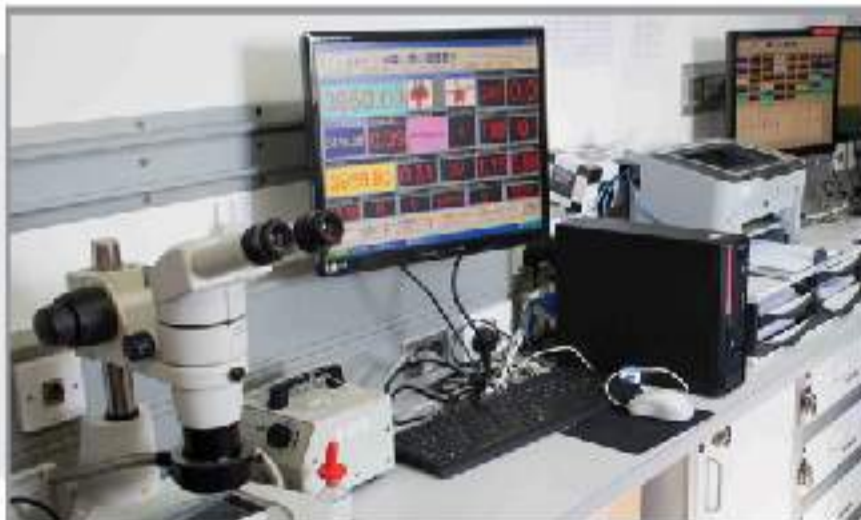
Online Computerized Mudlogging Unit in Kailashtila-7
