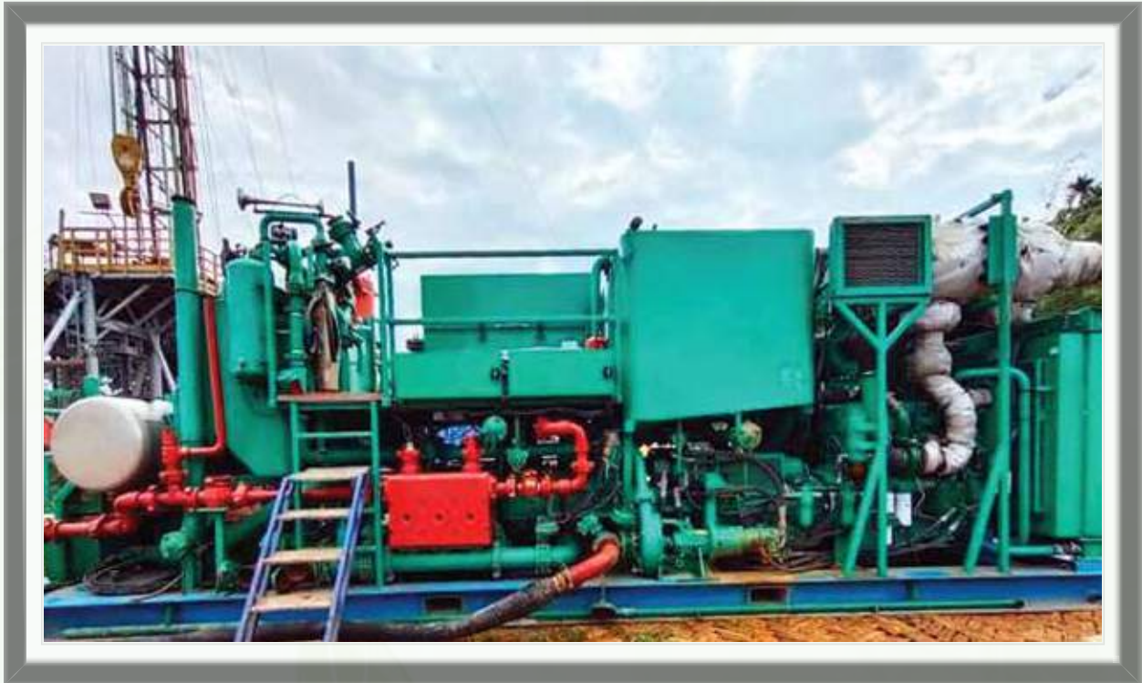
10,000 psi Cementing Unit (UEM, USA)
